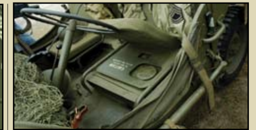
Gas tank beneath driver's seat.
