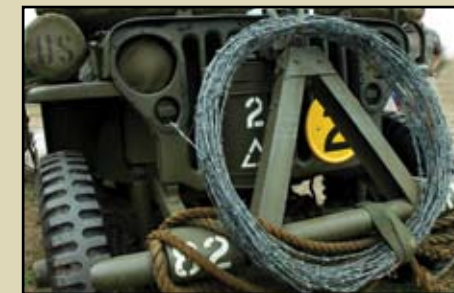
Tim equipped his jeep with an original tow bar. With these, one jeep could tow a whole series of jeeps together.
