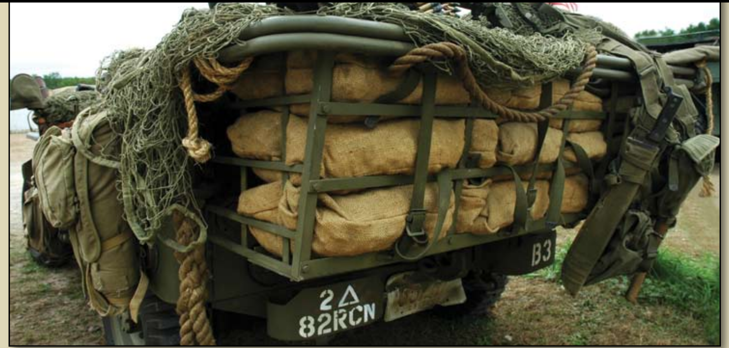
Tim added an original bundle basket on the tailgate. These were used to hold extra equipment and sandbags.
